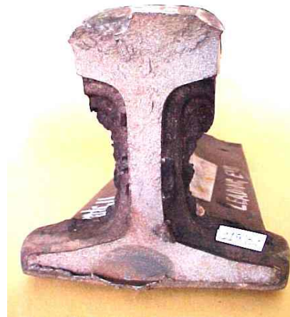
FIG. 51 : 421 - WELDING, THERMIT JOINT TRANSVERSE CRACK
