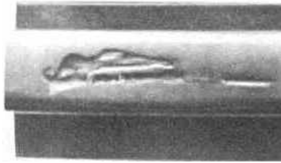
FIG. 36 : 1211 OR 2211 - HEAD, SURFACE, SHALLOW SURFACE DEFECT (FLAKING)
